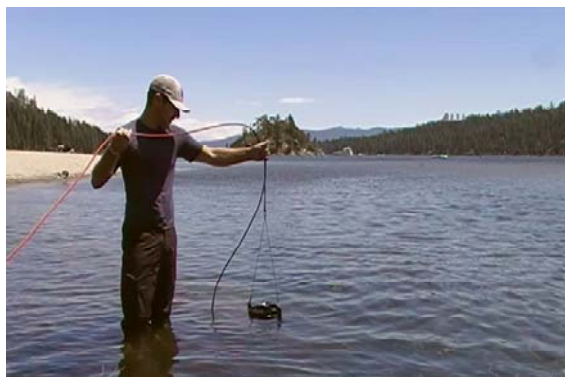
Figure 1. Using the Biospherical Instruments radiometer to collect UV and temperature data at Emerald Bay.
